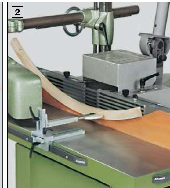
**1** Pressure module I and single wheel providing safe controlled pressure when edging curved workpieces.
